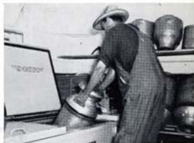
THE ELECTRIC MILK COOLER. —Milk keeps sweet in a modern regulated dairy cooler; 1 kilowatt-hour will cool 10 gallons of milk a day.
