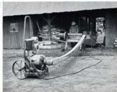
THE ELECTRIC SAW. —It saws up a cord of wood for as little as the cost of 2 kilowatt-hours, saves arm ache, time and money.
